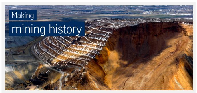
At 9.30pm on 10 April 2013, Rio Tinto Kennecott's Bingham Canyon Mine experienced the largest slide in mining history. Preparation for the slide had begun months in advance, after advanced geotechnical equipment identified increased movement in the north-eastern wall of the pit, and the company started to relocate and close buildings, access roads and equipment. Employees were moved out from the bottom of the pit before the 135 million tonne slide began, and not a single person was injured.
