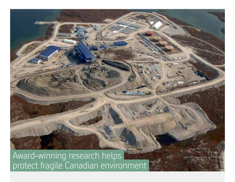
Waste rock contains sulphide minerals that, when exposed to air and water, can result in poor quality drainage. If not managed properly, the drainage can harm fish and aquatic life long after a mine has closed.
