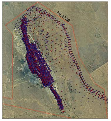
Open holes (blue); cored holes (red) Figure 3 Drill collar locations
