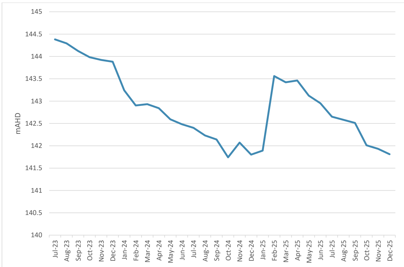
Figure 1: Groundwater level at bore PZ09MEJ004 (21.738953 S, 116.262437 E)
