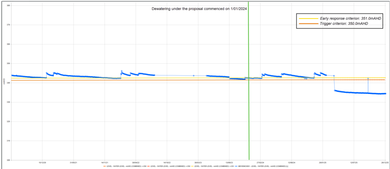
Figure 29: Groundwater level at MB19SMC0001- 2020 to 2025
