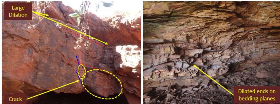
Figure 17 – Brow on the left with some structures and defined blocks (yellow ellipses) pointed out. Right hand side photo of the bedding condition on the walls just inside the cave entrance
