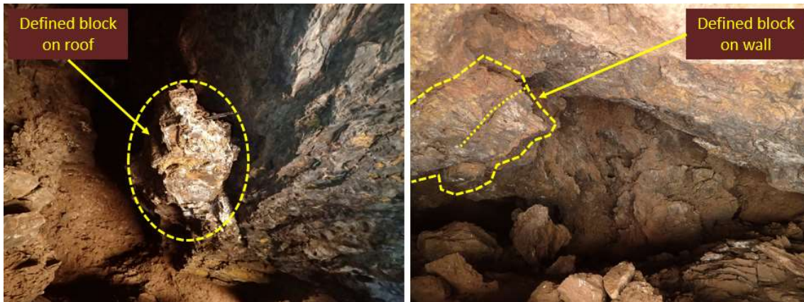
Figure 5 – Both photos indicate defined blocks in the cave. Take note that they are not loose
