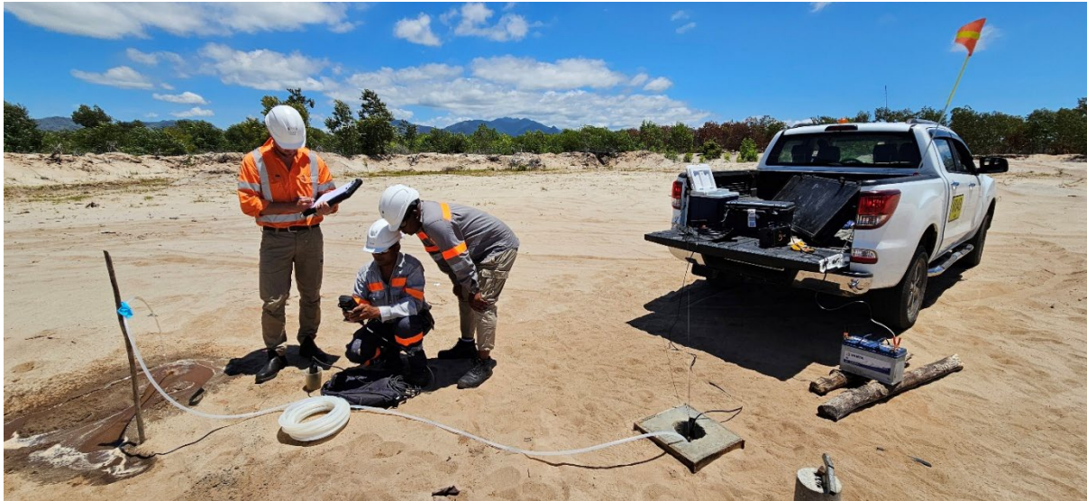
Figure 3-6 Set up of the submersible pump at GWBH10
