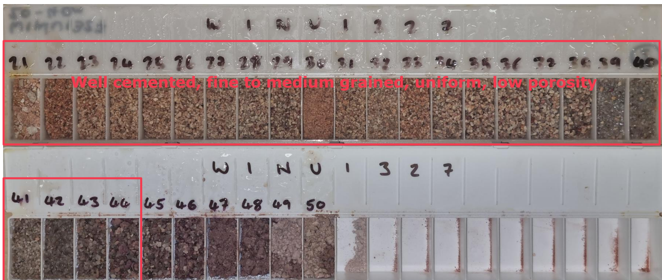
Figure 3-2: WINU1327 infiltration bore drill chip samples from Pond 1
