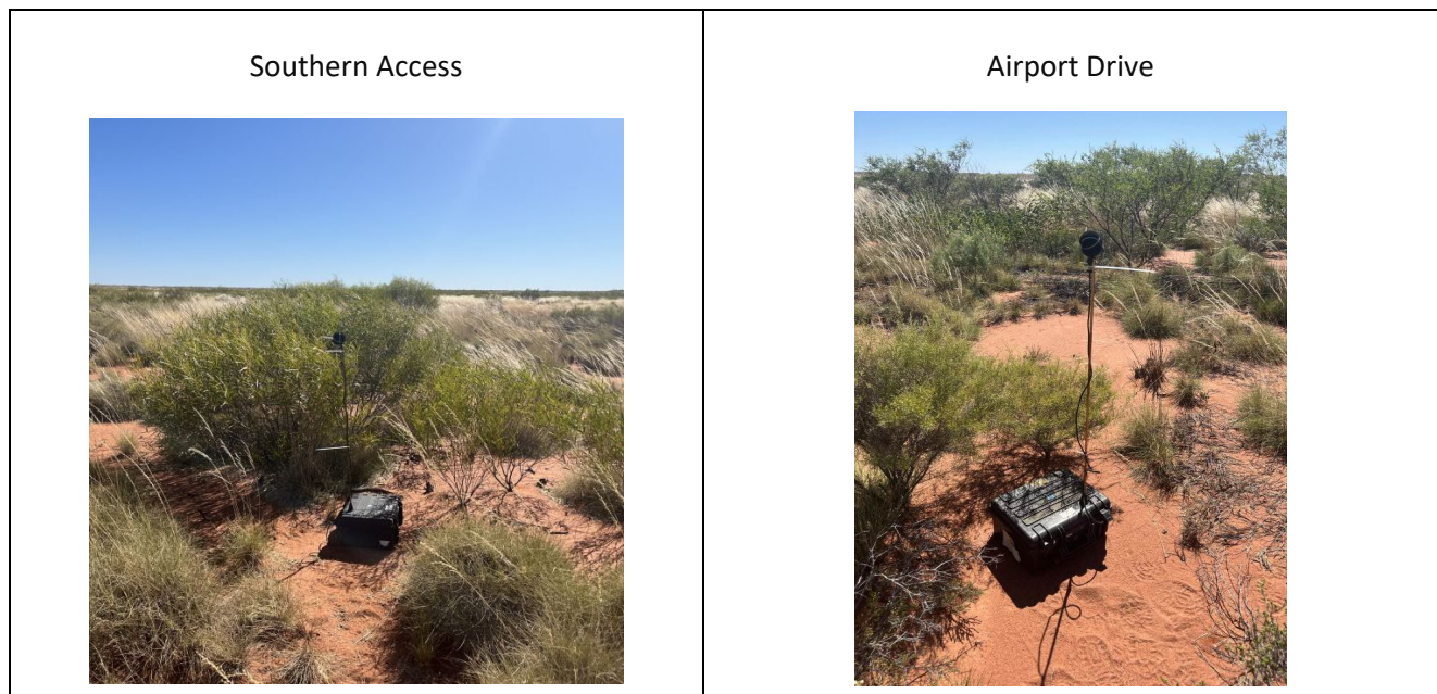
Figure 2-1: Ambient Noise Logging Equipment Installed
