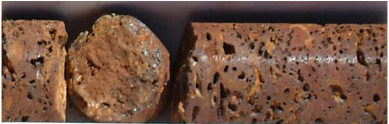
Plate 5.3: Example of a drill core from the Pilbara showing fractures and cavities typical of subterranean fauna habitat.
