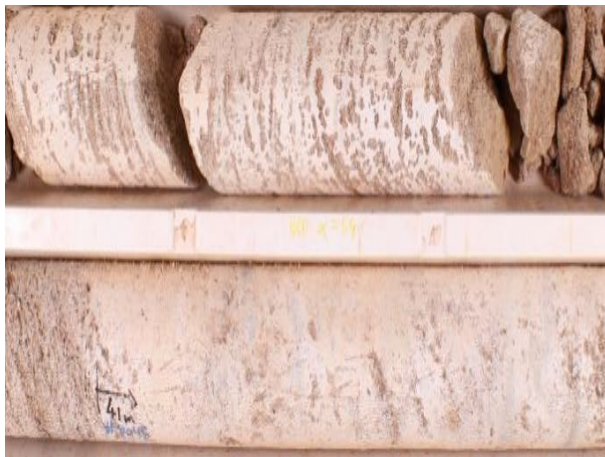
Plate 5.4: Site WINU0059 at approx. 41 m: porous sandstone.
