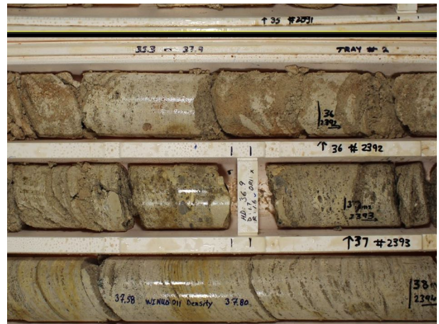
Plate 5.5: Site WINU0011 at approx. 35 m: porous and fractured sandstone.
