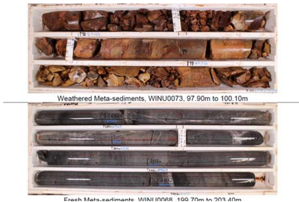
Figure 2.11: Core photo of weathered and fresh metasediments
